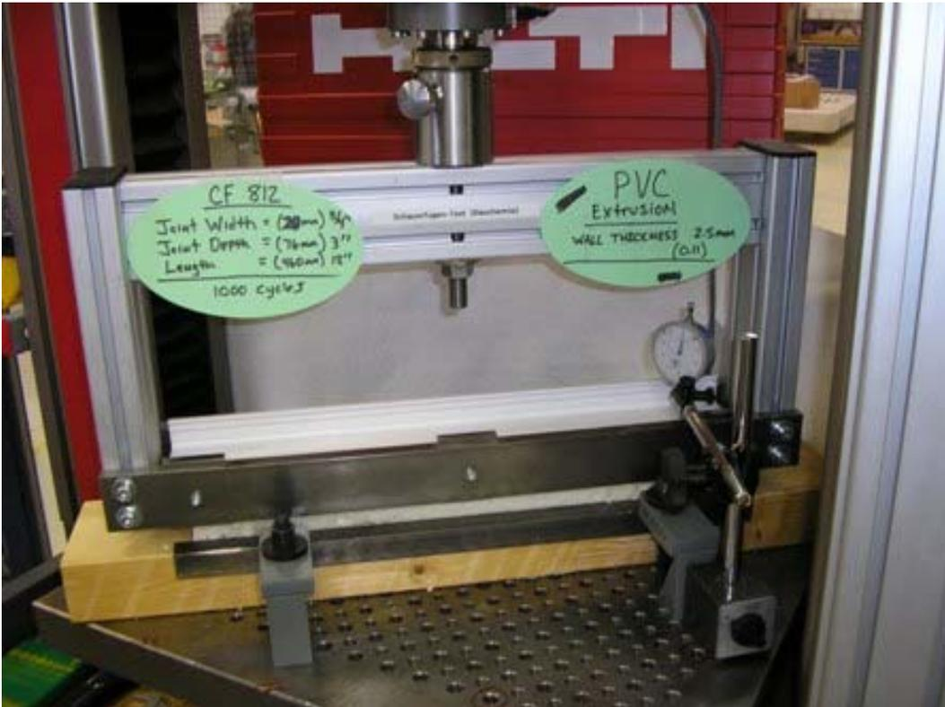
PVC window extrusion with CF 812 between wood and PVC mounted in the tensile strength machine simulating joint movement.
