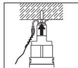
4. Locate the nail, compress the tool, pull the trigger and the fastening is complete
